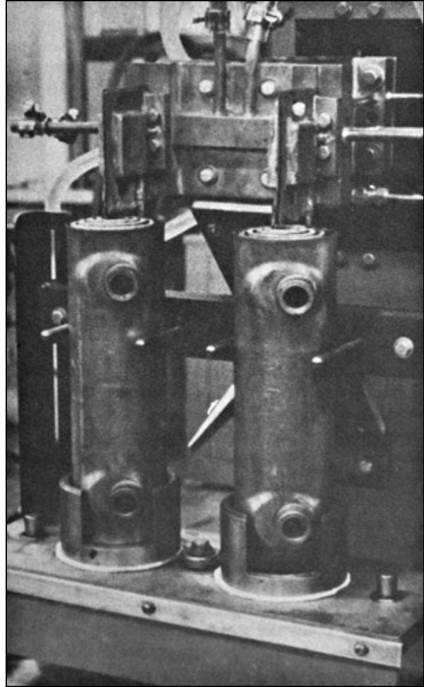
*Figure 7: Heavy malleable steel headers are brazed to copper bearing steel tubes for a manufacturer of radiators.*
