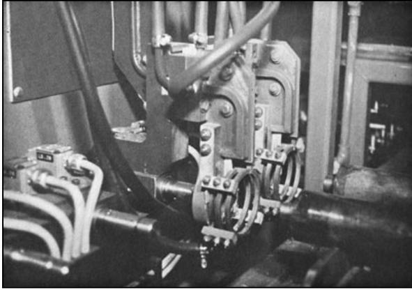
*Figure 6: Brazing station on a robot-operated line making office copier rolls. Brazing and cleaning are done in-line.*
