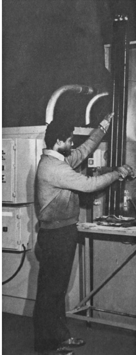
Figure 3 generator, operating a 450-kHz produces 1800 parts per hour with an automatic stripper removing parts from the conveyor at the exit end.
